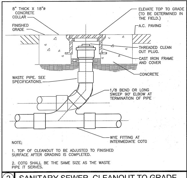
SANITARY SEWER, CLEANOUT TO GRADE<sub>NTS</sub>
