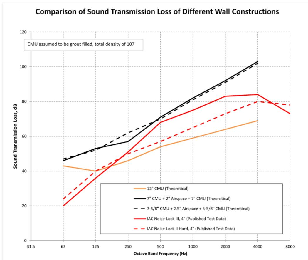
\* Theoretical assumes no edge damping, no insulation in airspace between CMU
