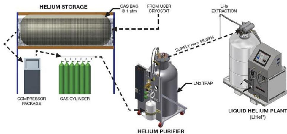
**Figure 6-1. Helium Recovery Concept Diagram Showing Components**
