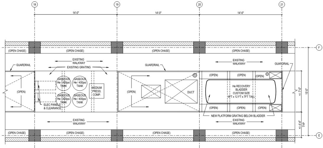
**Figure 6-2. Collection Bladder & Medium Pressure Helium Recovery**
